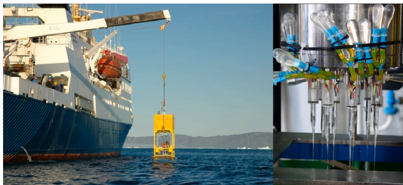
Fig. 3. Left: Recovery of deep sea lander for microprofiling after a completed mission. The electronics cylinder in the lower center of the yellow frame is mounted with an array of microsensors that were introduced stepwise into the sediment. Right: Close-up of electronics cylinder mounted with microsensors. The transparent bulbs are filled with oil that is squeezed into all sensor cavities when the pressure increases. After a 12-24 h long operation at the bottom, the ascent is initiated by release of ballast. Photos by S. Rysgaard & R.N. Glud, with permission. (For interpretation of the references to colour in this figure legend, the reader is referred to the web version of this article).
